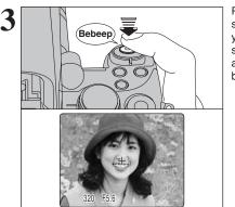
Press the shutter button down halfway. When a short double-beep is heard, the camera focuses on your subject. The AF frame on the screen becomes smaller and the camera sets the shutter speed and aperture. The indicator lamp (green) changes from blinking to lit.
